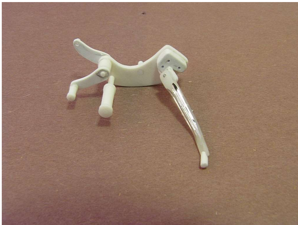
Figure 8 - left side footpeg, clutch pedal and kickstand
