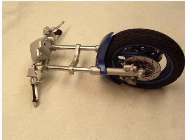
Figure 6 - Completed front fork.
