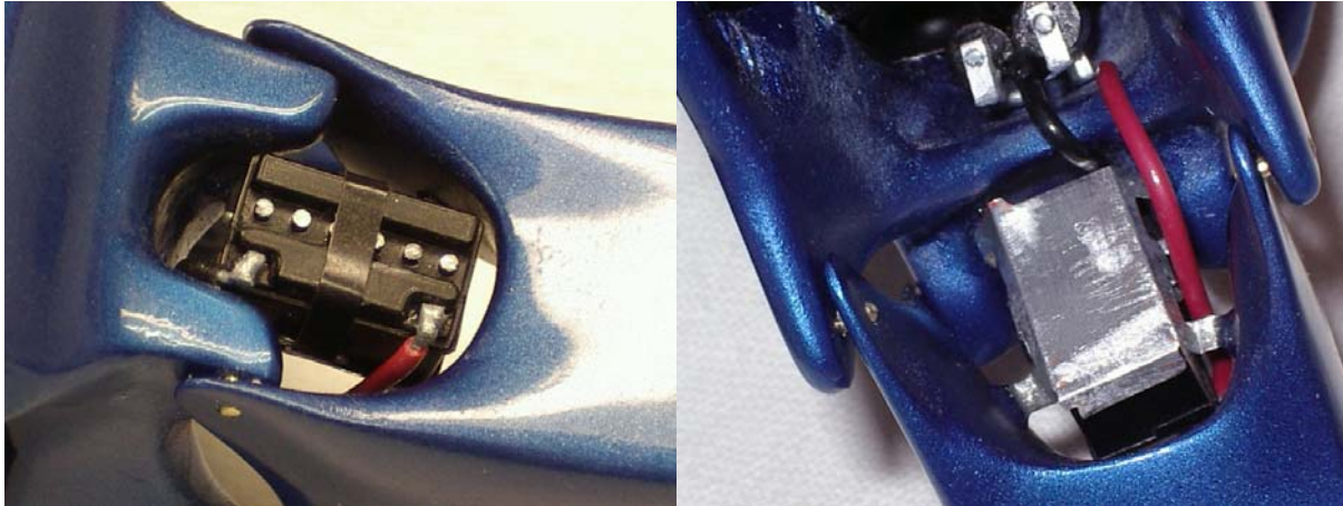
Figure 15 - Completed battery top view. Bottom view showing mounting pan/bracket and back end of ignition coils.
