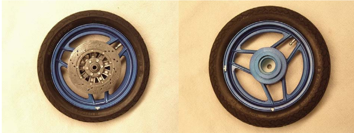
Figure 3 - Front (left) and rear (right) wheels showing wheel weights and air valves.
