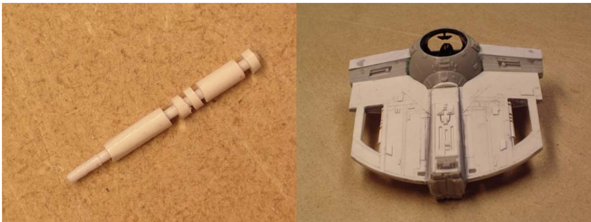
Figure 27 Detail part for the larger opening was made from styrene rod and tube. Small raised panels on the body and arms were made from 0.25 mm (0.010") and 0.50 mm (0.020") thick styrene. Right photo shows rear just before painting. Tamiya putty was used on the joints.
