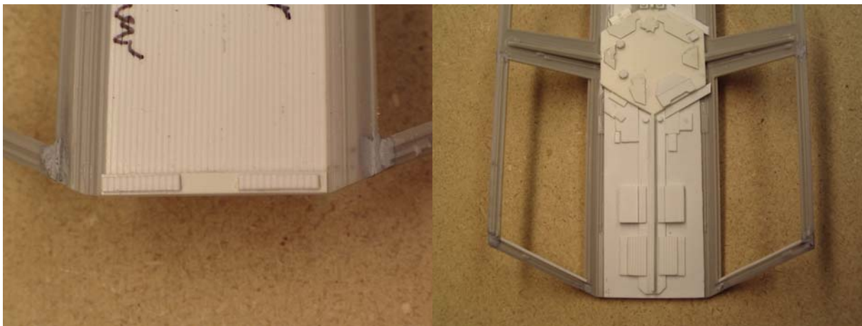
Figure 12 Rear part of wing were detailed with sheet styrene and some small pieces of the solar panel V-groove sheet. The inside of one wing could probably use more finer detailing.
