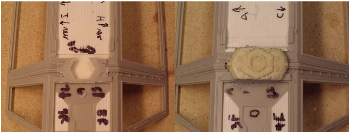
Figure 11 Outer details were filed off and then resin cast piece glued on.
