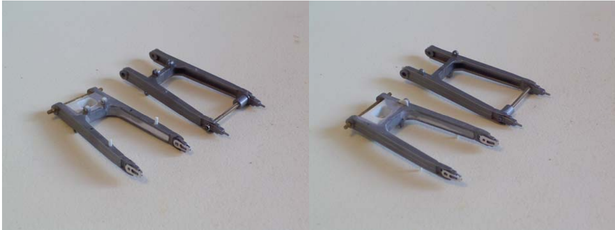
Figure 8 - Comparison of before and after modifications to swing arm
