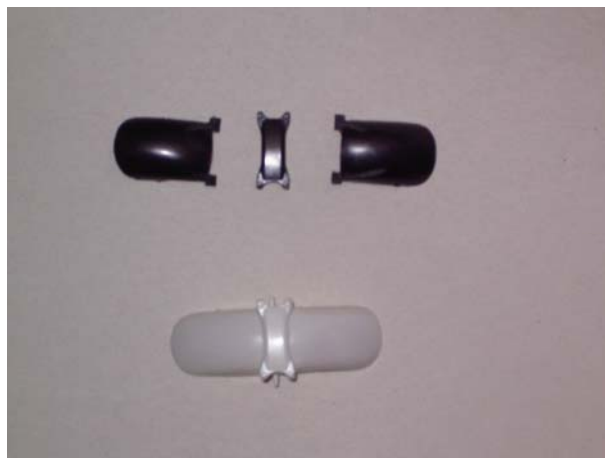
Figure 4 - Separated fork brace (above) and original (below)
