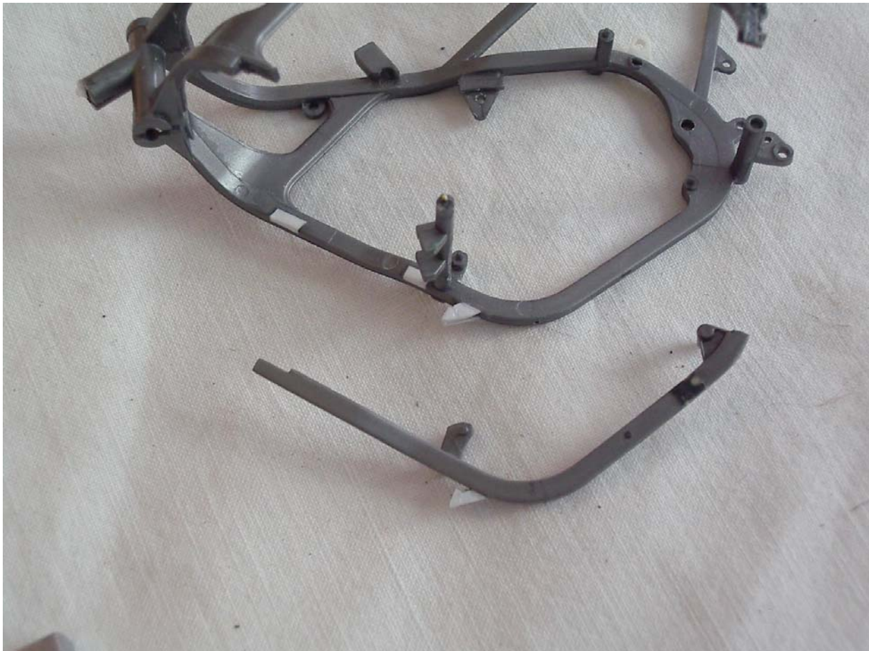
Figure 14 - Frame showing additional brackets and separated left side piece
