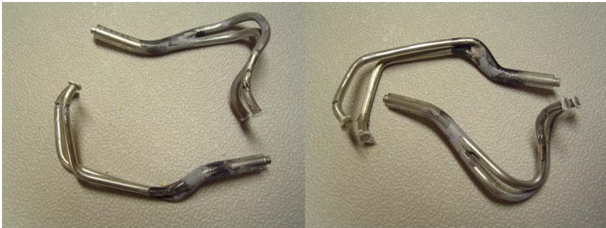
Figure 13 - Exhaust pipes from solder
